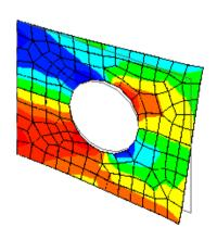
What: Display a contour plot of the Z component of displacement.
